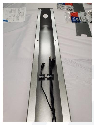
Peel backing off the cable mounting pad.
