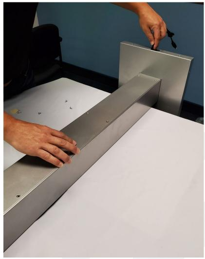
Slide the top panel back into the base, add and secure the screws. Please be careful not to pinch the USB cables and the power cable.
