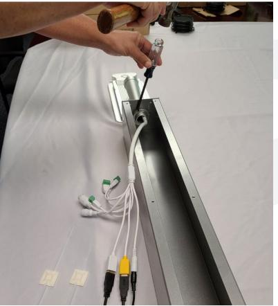
Feed the white cable connectors, two at a time, through the top hole of the Kiosk stand.
