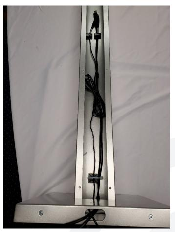
Wrap up the excess cords nicely and tie up at the bottom with a zip tie and cable tie mounting pad. Then put the excess (1-2 inch) cords through the hole in the base.
