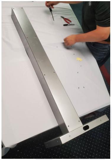
Find the side of the stand with 8 screws. Lie the stand down with that side face up and remove the screws. Then, remove the top panel and place it to the side.
