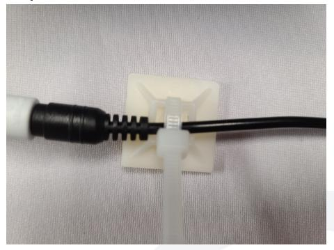
In another zip tie and cable mounting pad, secure the male end of the power cord. Cut excess zip tie.
