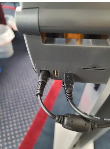
Plug in power connector (from back of stand) and (supplied) 1 FT. USB Cable from back of printer to the USB port on the back of stand. Push power button on front control and hit the feed button to feed label.
