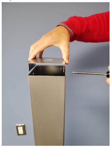
Remove the top piece of the stand by unscrewing the two screws located at the top right and left of the stand.
