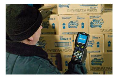
condensation is present. Condensation forces workers to enter data manually and prevents them from taking advantage of on-screen prompts. Heaters are therefore essential for cold-environment use. Internal heaters are recommended if computers will be consistently used at temperatures of 14°F (-10°C) and below, or will frequently move in and out of cold areas.
