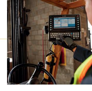
The ultimate ultra-rugged Android (VC80x) and Windows 10 (VC80) touch vehicle mount computer for the most extreme environments.
